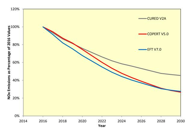
Figure 2: Relative Change in NOx Emissions Over 16 Years Assuming Constant Traffic Flows on a Nominal Road
