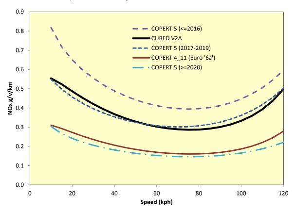
Figure 1: NOx Speed-emission Curves for Euro 6 Diesel Cars from Three Emissions Models
